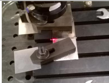
Fig.10: Experimental clamping setup for Filler material
