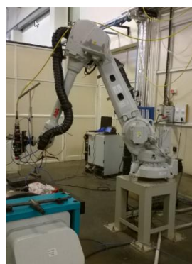
Fig.3 laser welding robot
