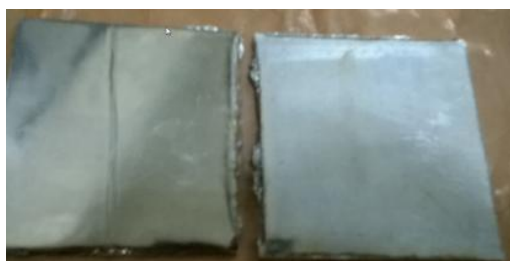
Fig.6: Joint after Weld
