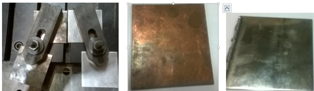
Fig.5 Fixture setup and raw copper plates before and after plating
