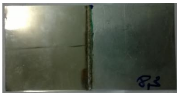
Fig.9: Pulse: ON/OFF 8/3 ml-sec
